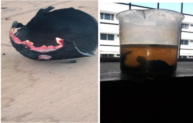
Fig.1: (a) Burned coconut shell, (b) Burned coconut shell was soaked in NaOH
